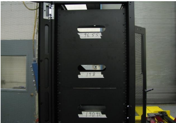
UUT weight distribution top portion in lbs
